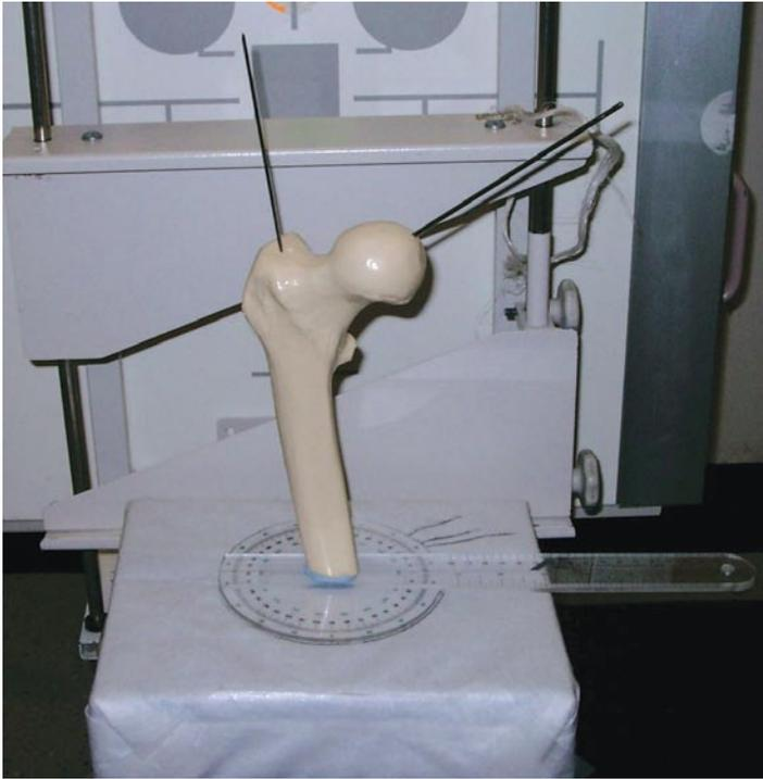
**Figure 3:** Saw bone model mounted on goniometer.
