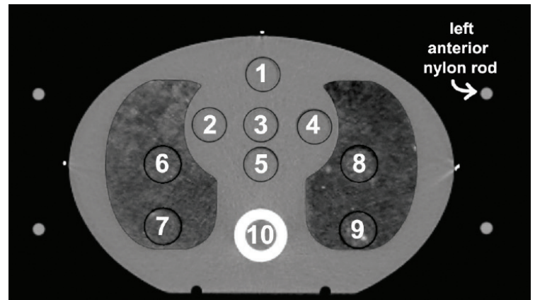
Figure 3: Sample CT scan of the central slice of the phantom with radiographic markers, numbering system for internal rods and the external left anterior nylon rod (LANR).
